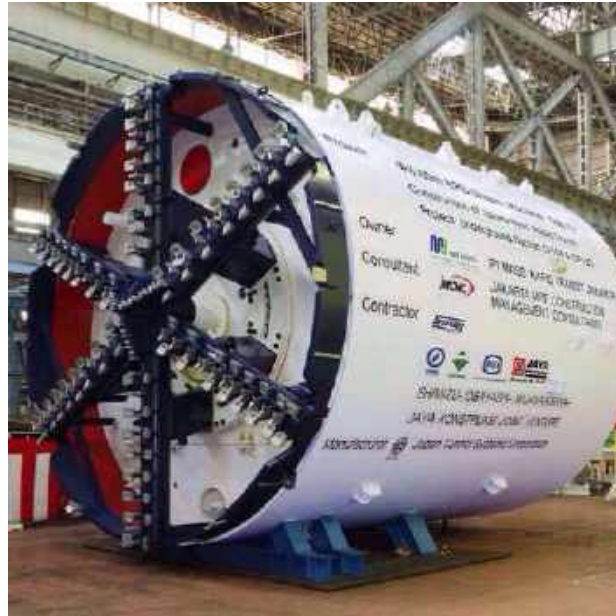
Gambar 2.12 Cutter Head TBM
